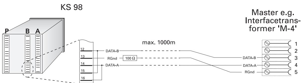
If an RGND connection is required with a setting for RS485, a 1000Ω resistor must be fitted between terminal 13 (GND) and terminal 5 on the interface transformer.
