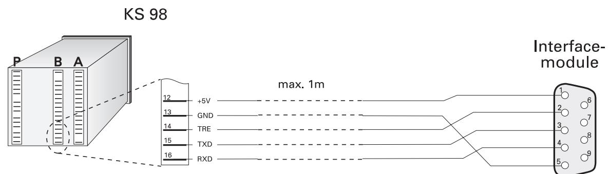
The connector is designed for using interface cable 9404 407 50011 for connection to the interface module. In the interface module, the connections of the instrument interfaces are galvanically connected with the bus interface and galvanically isolated from the supply voltage.
